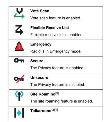
In the absence of a repeater, radio is currently configured for direct radio to radio communication.
