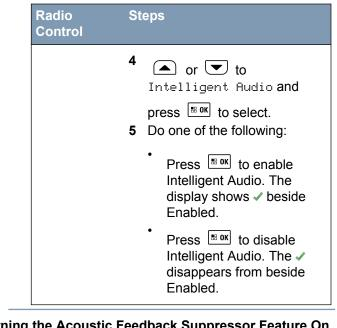
Turning the Acoustic Feedback Suppressor Feature On or Off
