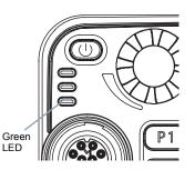
**NOTE:** The green LED lights up while the radio is transmitting and blinks rapidly when the radio is receiving a privacy-enabled call.
