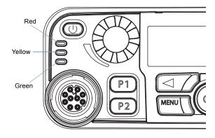
**Blinking red** – Radio is receiving an Emergency transmission or has failed the self-test upon powering up.
