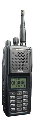
Equipped with an enlarged speaker, dual microphone, AMBE+2™ and Active Noise Cancellation, the XG-75Pe delivers clear audio despite noisy, congested environments.
