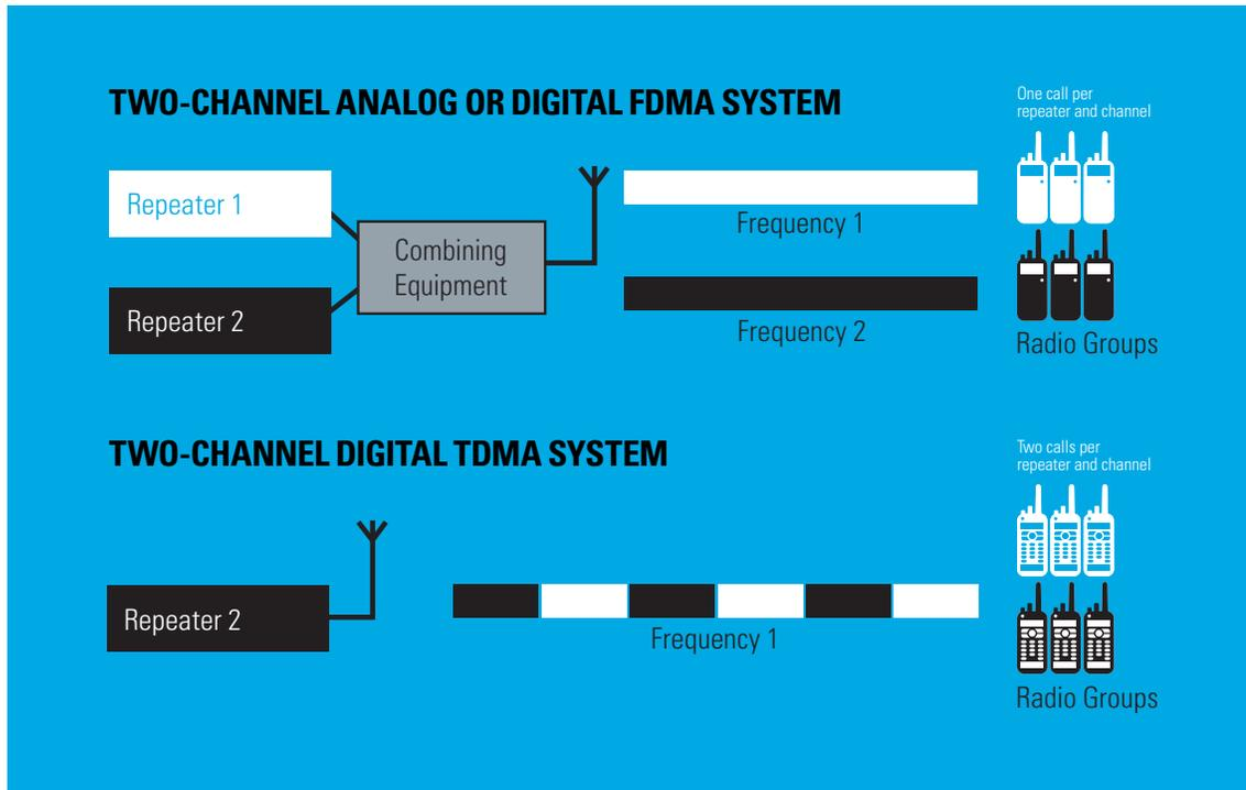
TDMA saves licensing and equipment costs by enabling the equivalent of two 6.25 kHz channels within a single licensed 12.5 kHz channel
