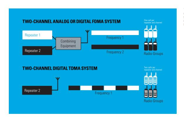
TDMA saves licensing and equipment costs by enabling the equivalent of two 6.25 kHz channels within a single licensed 12.5 kHz channel
