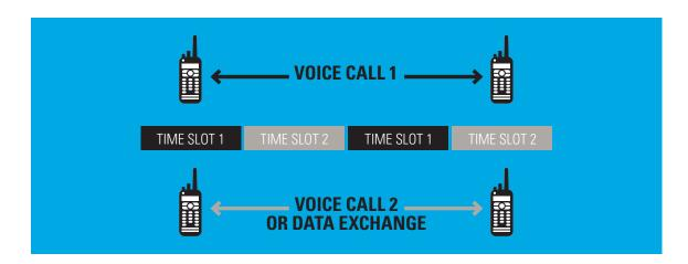
TDMA divides a 12.5 kHz channel into two alternating time slots to achieve 6.25 kHz equivalent spectral efficiency when used with a repeater.
