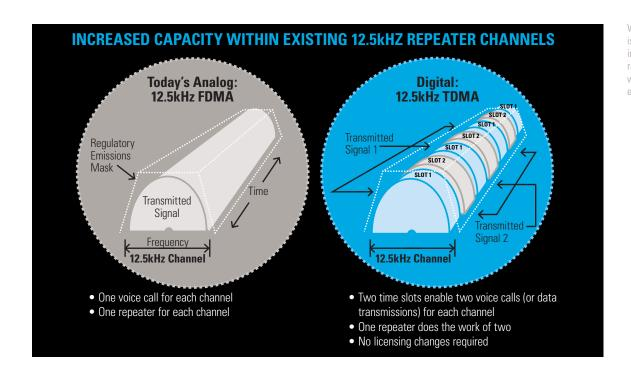
When FDMA technology is used to split a channel into two sub-channels, the resulting signals must still fit within the channel's required emissions mask
