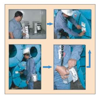
transfer and shipping of finished products over both land and water has been optimized. Product weight is automatically captured and printed on the labels.
