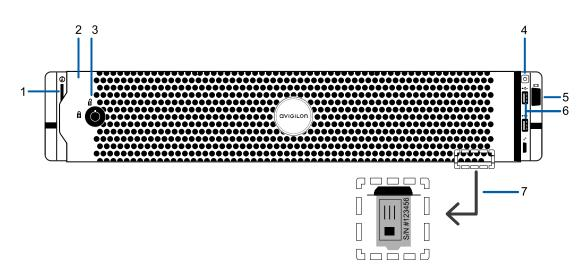
Figure 1: Front view of AI NVR Standard showing information tag (accessible after removing front bezel)
