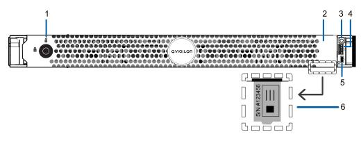
Figure 4: Front view of AI NVR Value showing information tag (accessible after removing front bezel).
