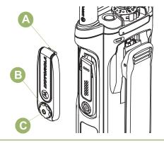
2 Rotate and lift the connector cover to disengage it from the radio.
