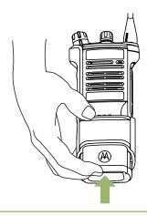
**4** Push at the bottom of the radio until the radio is released from it.
