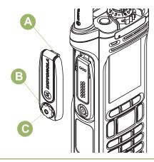
2 Rotate and lift the connector cover to disengage it from the radio.
