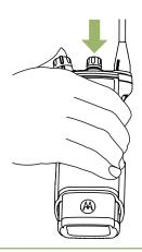
3 To remove the radio from the carry holder, place the tip of your fingers on the ledge of the carry holder.
