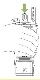
**3** To remove the radio from the carry holder, place the tip of your fingers on the ledge of the carry holder.
