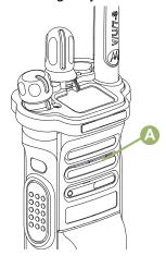
Your radio is designed to be submerged to a maximum depth of 2 meters, with a maximum submersion time of 4 hours. Exceeding either
