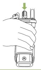
**3** To remove the radio from the carry holder, place the tip of your fingers on the ledge of the carry holder.
