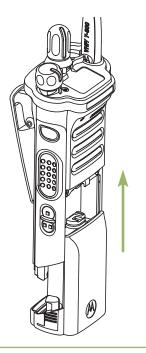
**Note:** When removing the battery, ensure that the radio is turned off.
