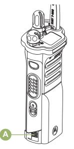
2 To remove the battery, squeeze the release latches (A) at the bottom of the battery until the battery releases from the radio and remove the battery from the radio.
