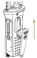
2 Use a flat-bladed object to press the belt clip tab away from the radio. Then, slide the clip downward and away from the radio to remove the clip.
