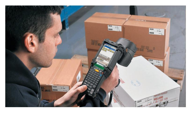
in a receiving scenario, incoming shipments are automatically identified as they pass through the dock doors. Shipments are verified against the purchase order and instructions to the worker are sent out — back orders are cross docked to shipping, damaged goods are staged for return, and shipments bound for inventory are staged for put-away.
