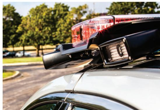
Motorola offers an ALPR Expansion Board for the MW810 that supports up to four Slate™ digital ALPR cameras from PIPS Technology. Working together, Motorola and PIPS have created an ALPR solution with unparalleled power, intelligence, and flexibility – and without the footprint of a separate ALPR processor.
