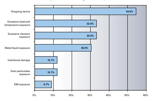
The value of ruggedized devices is that they are designed to protect the most sensitive parts from likely damage:
