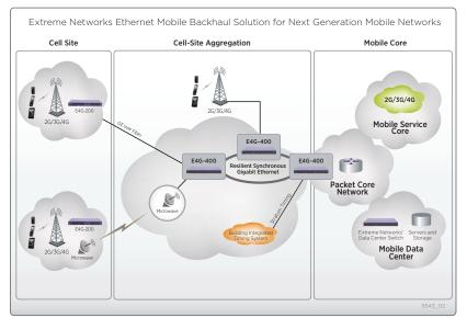
Figure 1: Typical Network Architecture for Wireless Backhaul
