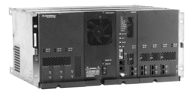
The ASTRO-TAC 9600 comparator is a digital Simulcast<sup>™</sup>/ Voting comparator for use with Motorola's Project 25 compliant system ASTRO®25
