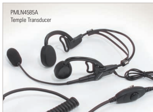
Temple Transducer Innovative headset design lets users receive audio without covering their ear.
