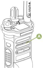
Your radio is designed to be submerged to a maximum depth of 2 meters, with a maximum submersion time of 4 hours. Exceeding either maximum limit may result in damage to the radio.
