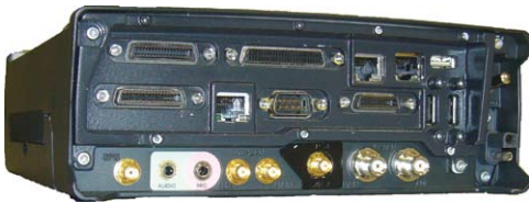
A fixed-mount workstation has a large number of ports for external devices.
