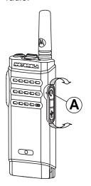
Lift the flap of the Audio Jack cover. Align the indicators (A) on both the connector and housing, then push until it fits in properly.
