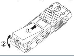
2 To attach battery cover, align it in place and slide the battery latch until it snaps into place. Slide battery latch into lock position.
