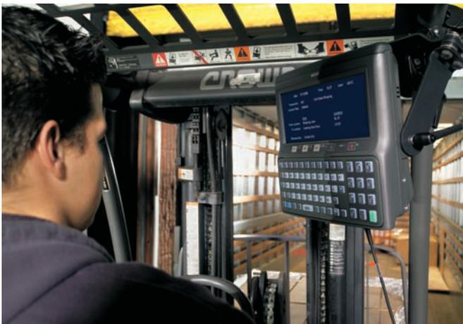
And even in the far corners of your warehouse storage areas where lighting may be less than optimal, the backlit keyboard ensures ease and accuracy of data entry. Features combine to allow the VC5090 to deliver the reliable performance you need to keep your receiving and put-away operations at peak productivity.
