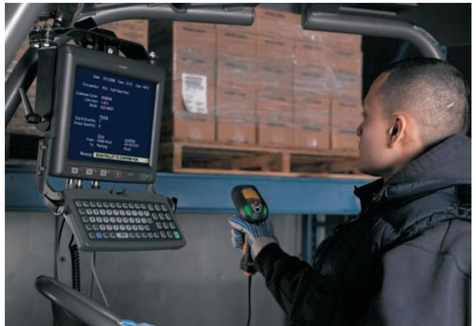
well spaced keys on the full QWERTY keyboard. And while the VC5090 receives its power from the forklift battery, an optional internal uninterruptible power supply (UPS) assures continued operation even on gas-powered trucks. With this option, forklift operators never need to power off the VC5090 and reboot, even when the forklift battery is changed (usually once or twice every eight to twelve hour shift).
